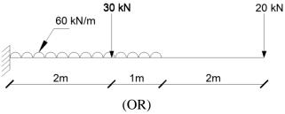
4. (a) For the cantilever beam shown in figure plot the SFD and BMD.
