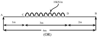
8. Find the deflection at points C and D of the beam loaded as shown in fig below, by moment area method. Given E=200 GPa, I=66.67x10<sup>6</sup> mm<sup>4</sup>.
